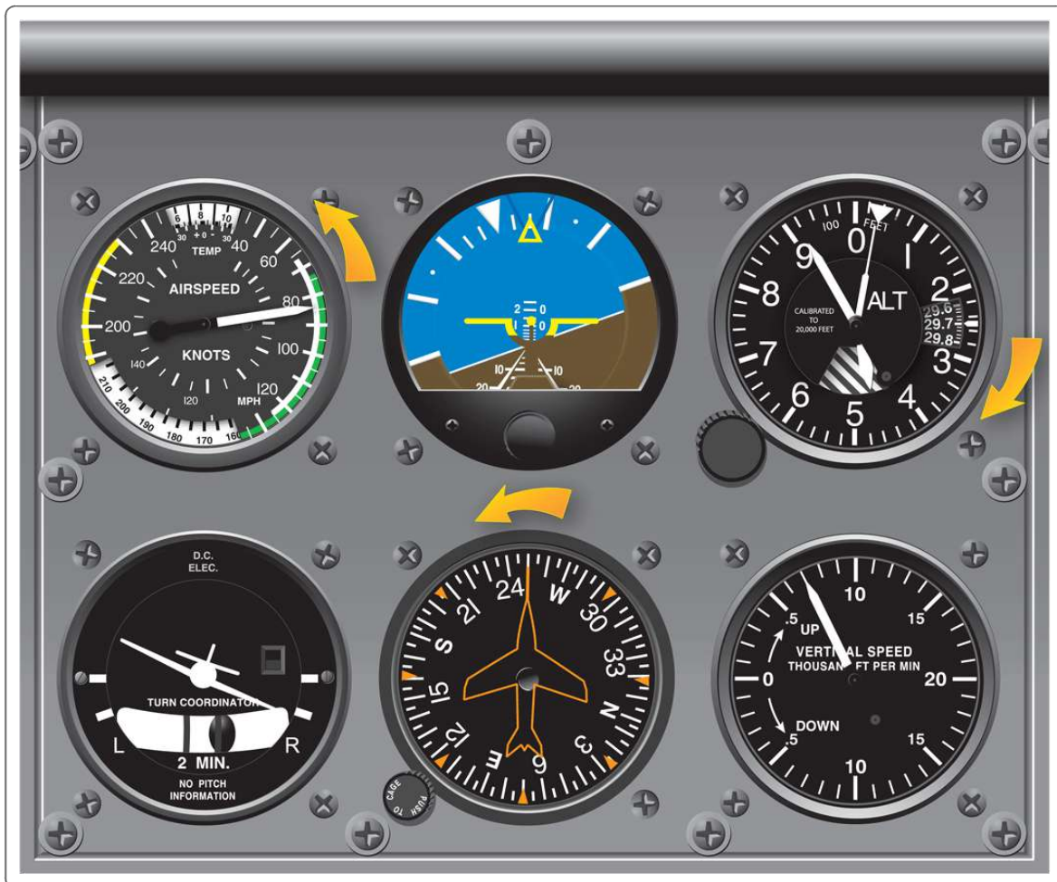
Figure 147. Instrument Sequence (Unusual Attitude).
