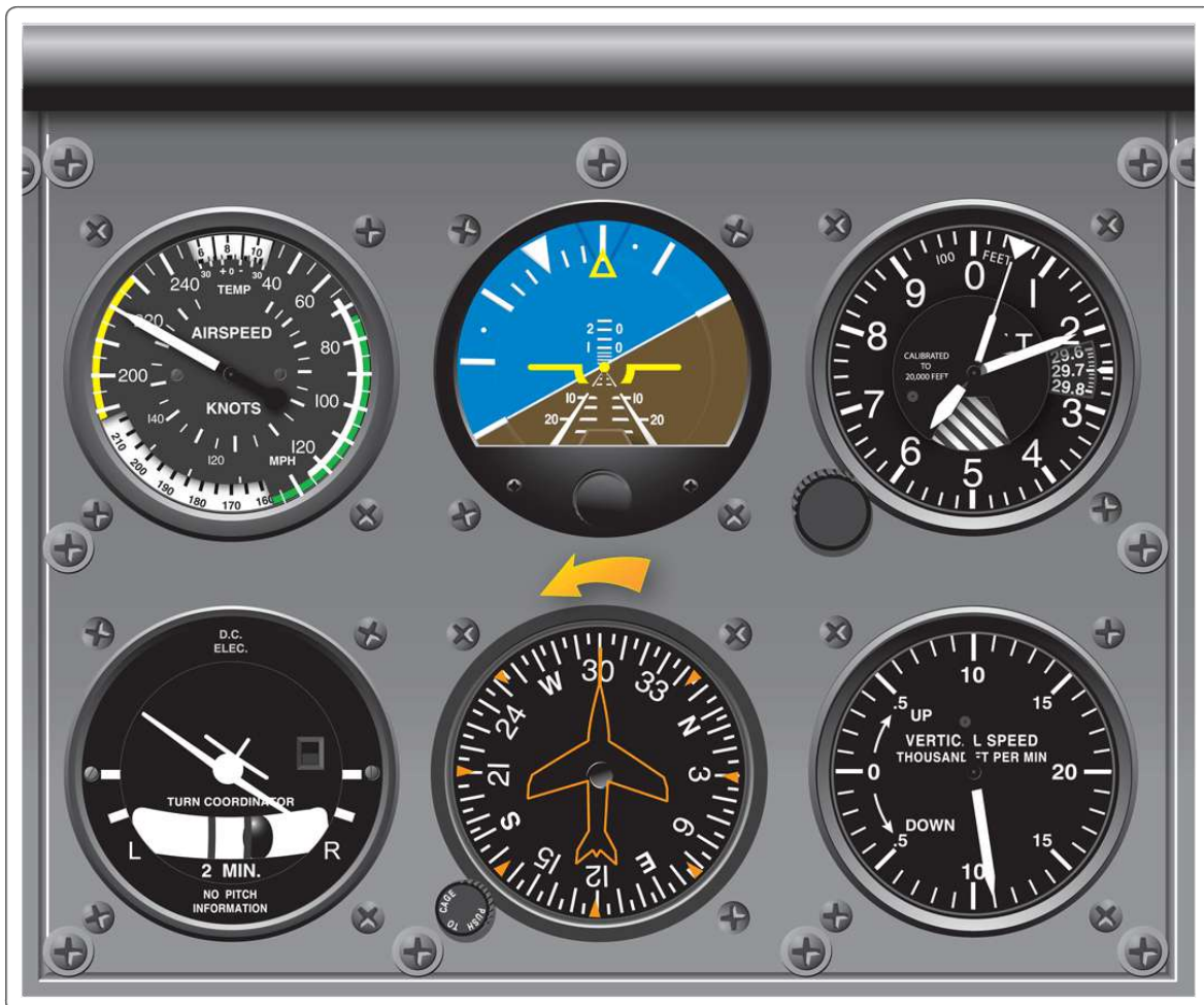
Figure 145. Instrument Sequence (Unusual Attitude).
