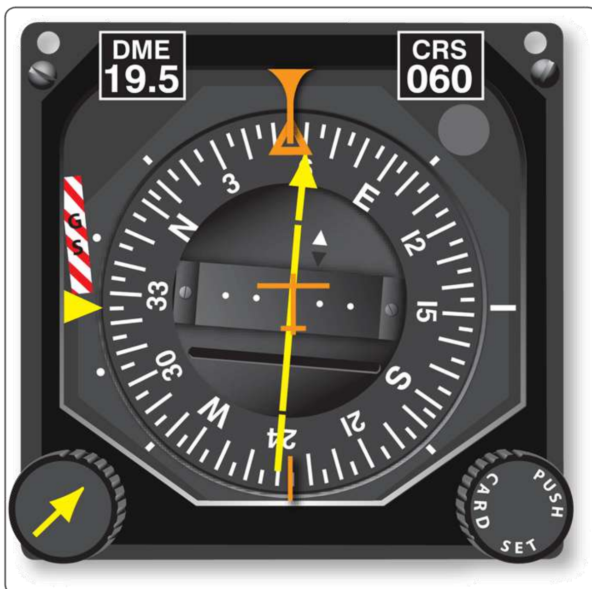
Figure 113. Aircraft Course and DME Indicator. ©ASA
