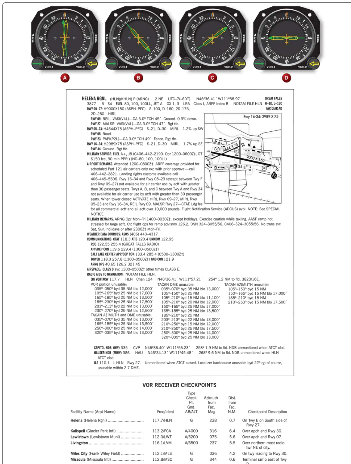
Figure 76. VOR Indications and Excerpts from Chart Supplement (HLN).
