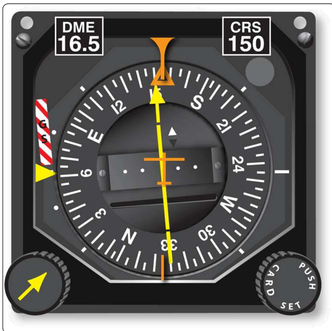
Figure 114. Aircraft Course and DME Indicator. ©ASA
